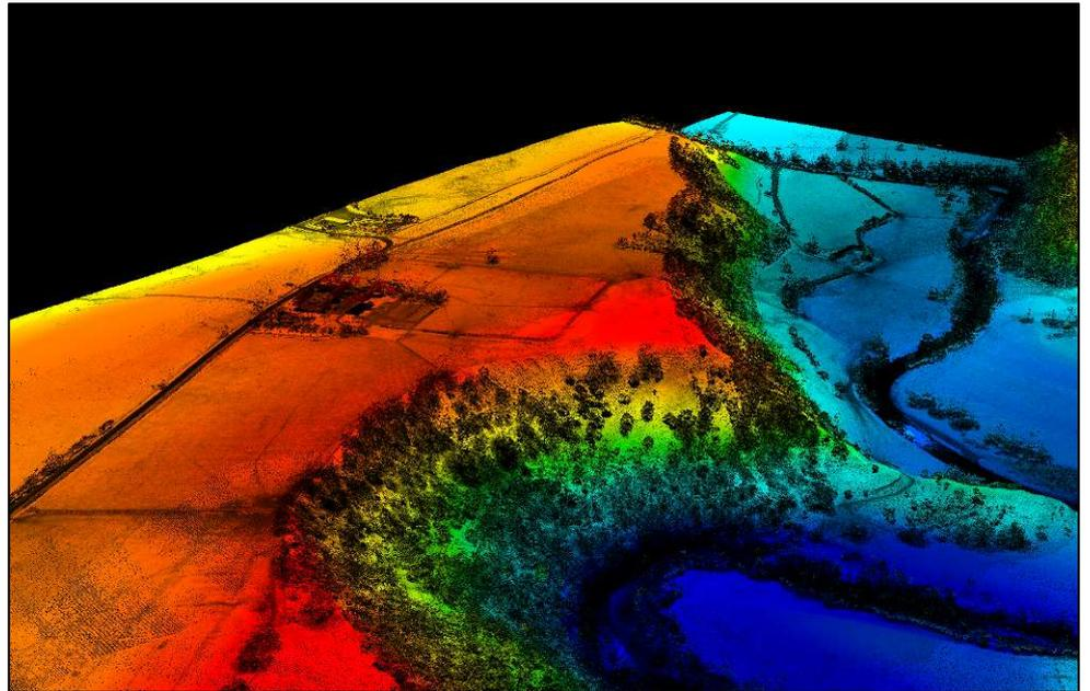
**Figure 1: Cultural heritage can now call upon three-dimensional techniques such as laser scanning to inform conservation at a variety of scales, as seen here in an airborne laser scan of Birdoswald Roman Fort (above) and a terrestrial laser scan of an archaeological dig at the same site (below).**
